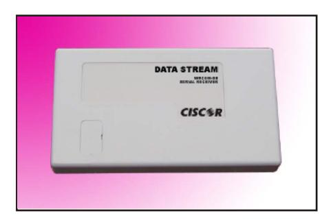
The WRCOM-DS wireless serial receiver is the gateway that uses reliable frequency-hopping, spread-spectrum technology to decode radio frequency (RF) transmissions from end devices and high-power repeaters. It then outputs the decoded data to the central computer. It is connected to a USB port on the central computer and appears as a COM port in the software. The unit comes with an RS232 serial DB9 connector and a plug-in transformer ready to install. An RS232 to USB converter is required.
